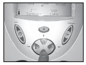
2. Press the Frequency button to select 1 or 3 MHz. When the button is pressed, the frequency will toggle from 1 to 3 MHz and back again as long as the button is being pressed.
