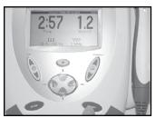
7. Press the START button. The unit will beep 5 times and the ultrasound power will distribute the selected output.
