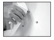
7. Line up the screw heads with the holes on the mounting brackets, and slide the unit down slightly until the screw heads are securely fastened to the mounting bracket.
