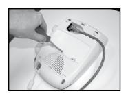
1. Locate the battery access door at the bottom of the unit and loosen the screw with a regular screwdriver.
