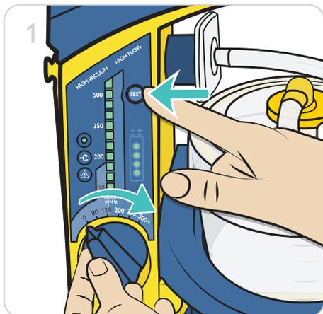
1. Press and hold the Test Button while turning the Operating Knob to 500+ mmHg.
